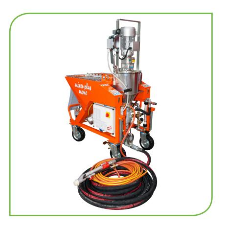
Single-phase (230 V) continuous mixing pump, ideal for spraying pre-mixed surface coatings containing lime, cement, finishing compounds, fillers, coloured compounds, adhesives, screeds, etc. and any product compatible with mechanical spraying.
